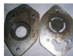
Carbonized valves and valve plates
