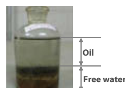
Free water in oil (Evaporator leak)
