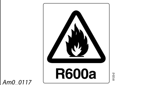
Fig. 6: Label on compressor for R600a
