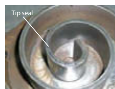
Melted tip seal; scored scroll spiral
