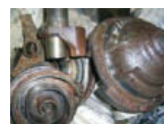
Mechanical parts and shell are rusty
