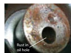
Inner surface of oil hole is plated by rust
